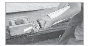
A wooden structure facilitates briquette extraction
