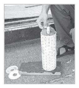
PVC pipe with holes that allow the water to escape
