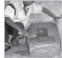
• Make sure the stove wall above the hole is not too narrow. It should be 5 cm high or more in order not to break easily.
