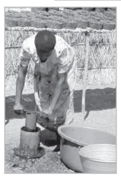
Pressing briquettes. Notice the briquettes drying at the top.
