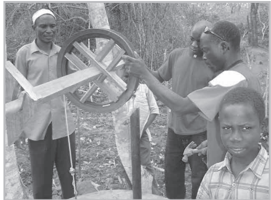
A wooden rope pump has been developed and is now made by local carpenters in Northern Mozambique
