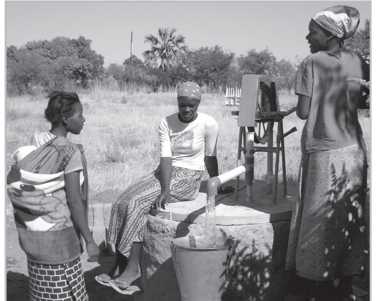
A locally made rope pump providing water in Zambia
